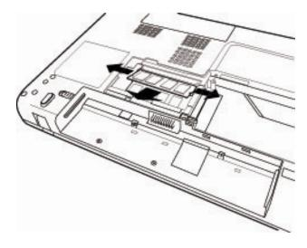
Figure 4-8 Removing the second memory
